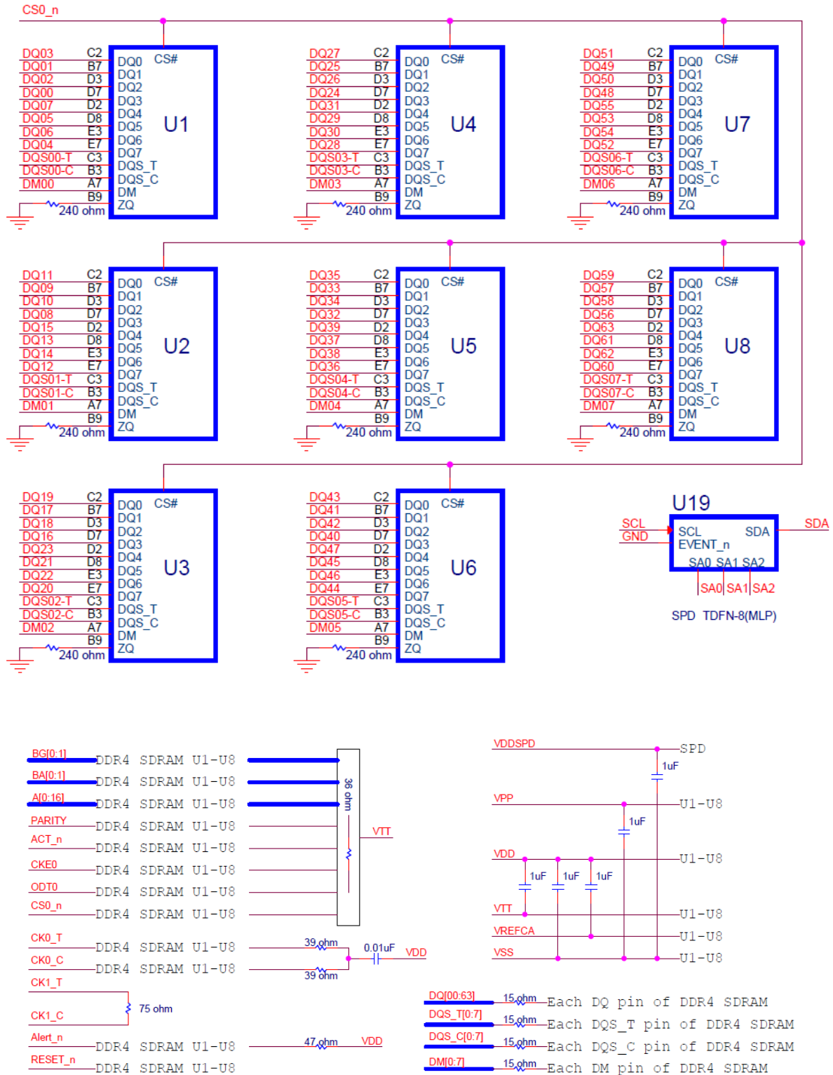
Figure 1 – Function Block Diagram_SCC16GU03H2F1C-32AA
